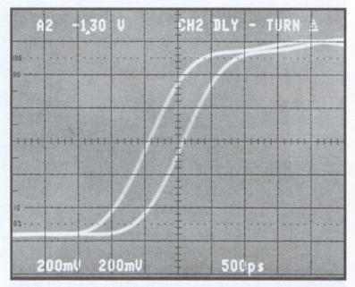
Adjustable delay increases accuracy. A frontpanel knob adjusts the Channel 2 delay to exactly match the Channel 1 delay from the probe tip.
