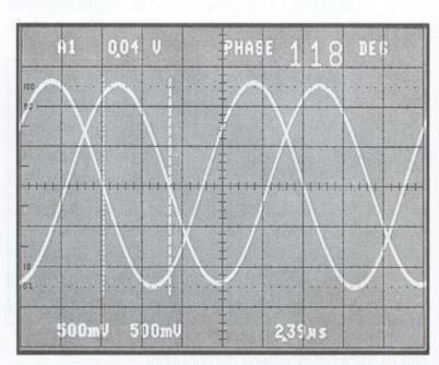
Measure phase shift in degrees or percent. The continuously-calibrated variable sec/div control sets one cycle (360° or 100%) to five horizontal divisions. The time cursors make phase and percentage measurements directly.
